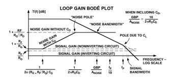
One disadvantage of this method of stabilization is the additional output noise and offset voltage caused by increased amplification of input-referred voltage noise and input offset voltage. The added dc offset can be eliminated by including  $C_D$  in series with  $R_D$ , but the added noise is inherent with this technique. The effective noise gain of these circuits with and without  $C_D$  are shown in the figure.
