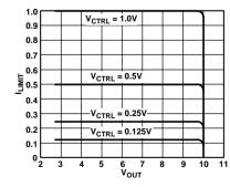
Figure 2. Current/Voltage Transition of the ADP3810 CCCV Charger
