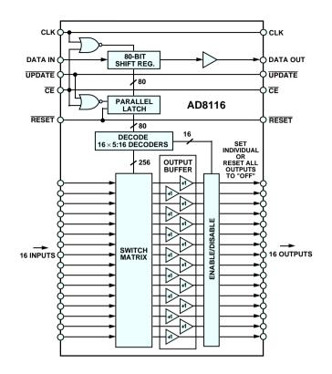
Figure 3. AD8116 functional block diagram.
