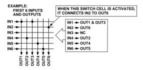
Figure 1. Non-blocking crosspoint switching.
