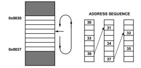
Figure 4. Example of modulo circular buffering.
