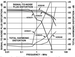
Figure 2. SINAD and THD vs. Signal Frequency
