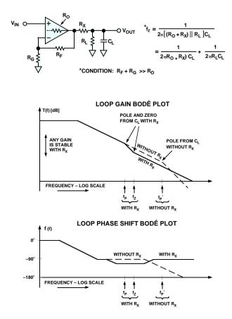
transfer function of the feedback network, thereby reducing the loop phase shift at high frequencies.
