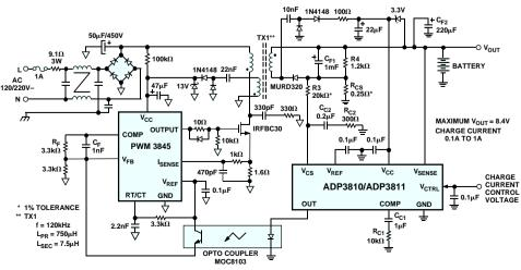
Figure 3. Complete Off-Line Li-Ion Battery Charger
