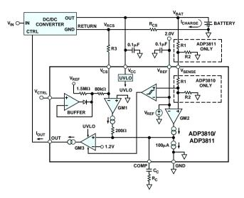
Figure 1. Block diagram of the ADP3810/3811 in a simplified battery-charging circuit.
